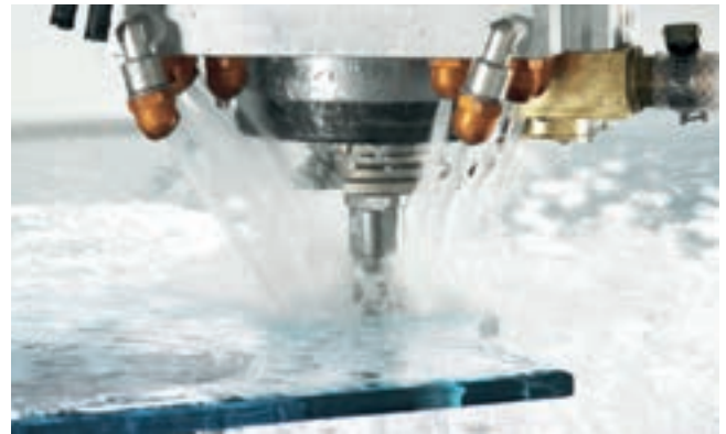
Boring from above.
