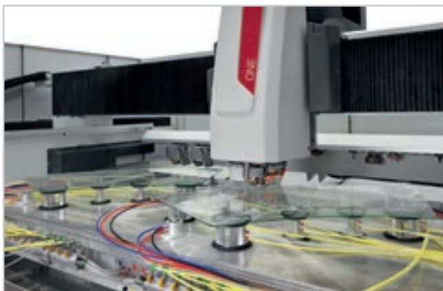
High speed grinding, particularly in demand in the automotive and household appliances sectors.
