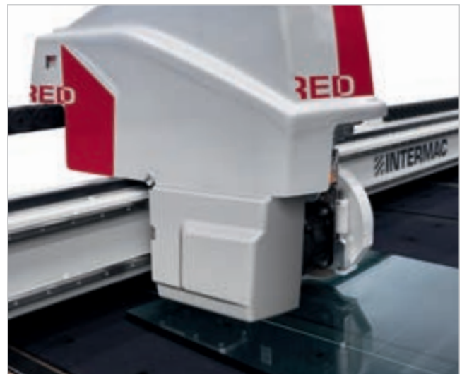
The roller-holder cones allow the cutting tools to be changed automatically.
