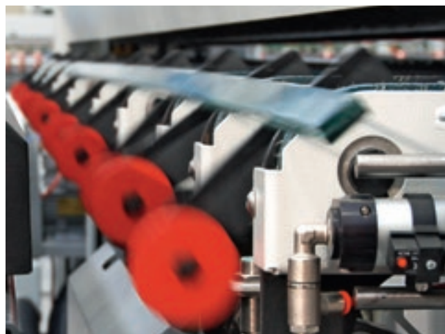
Cutting + automatic breaking + manual removal, 20 mm.
