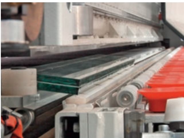
Cutting + breaking + standard removal, 60 mm.
