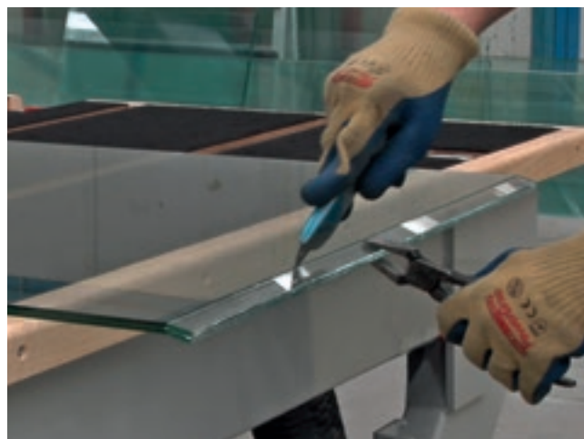
Cutting + automatic breaking + manual removal, 20 mm.
