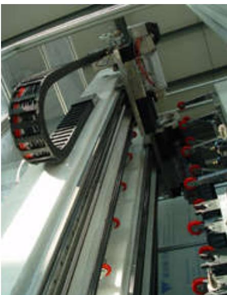
Glassman engineers designed double Y and V axis structure. Rigid structure make sure the high acceleration; Japanese servo motors drive the ball screw and slide way of the double Y and V axis to perfectly resolve the homocentric and exact location problem.
